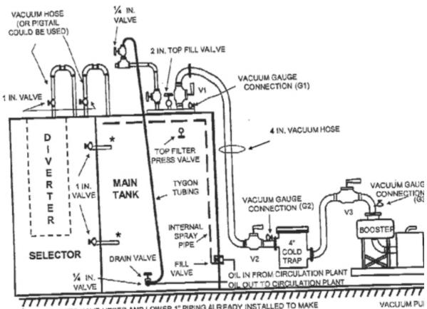
\* NEWER UNITS HAVE UPPER AND LOWER 1" PIPING ALREADY INSTALLED TO MAKE SELECTOR AND MAIN BODY COMMON (DO NOT LEAVE OPEN DURING OPERATION) VACUUM PUI
