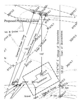
National Grid plans to interconnect via overhead conductor to the Village's proposed new metering pole from a new Company pole. The Company also plans to install a new in-line switch for reliability purposes.
