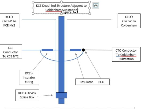
PCO is at the CTO end of jumper loop. OPGW PCO is inside the splice box. Dead-End Tower, Tower Hardware, Insulator Strings, conductor, OPGW and jumper loop between KCE NY2 and the PCO is owned by KCE (shown in blue). Conductor from the PCO and OPGW from the splice box owned by CHG&E (shown in Black)
