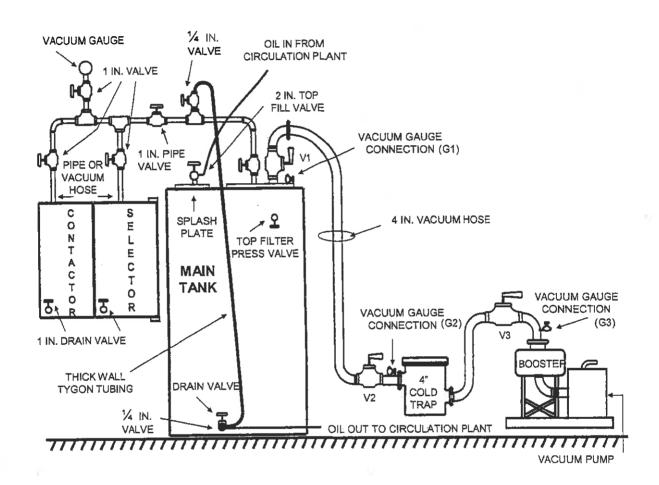
CE-ES-1003, INSTALLATION AND TEST SPECIFICATION FOR OIL IMMERSED POWER TRANSFORMERS, REACTORS AND REGULATORS
