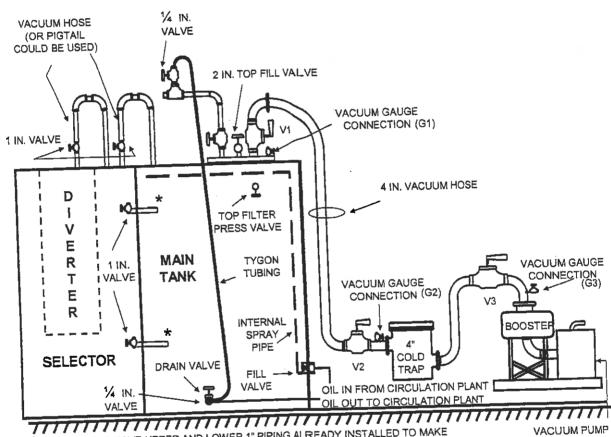
\* NEWER UNITS HAVE UPPER AND LOWER 1" PIPING ALREADY INSTALLED TO MAKE SELECTOR AND MAIN BODY COMMON (DO NOT LEAVE OPEN DURING OPERATION)
