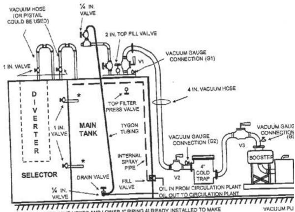
\* NEWER UNITS HAVE UPPER AND LOWER 1" PIPING ALREADY INSTALLED TO MAKE SELECTOR AND MAIN BODY COMMON (DO NOT LEAVE OPEN DURING OPERATION) VACUUM PUI
