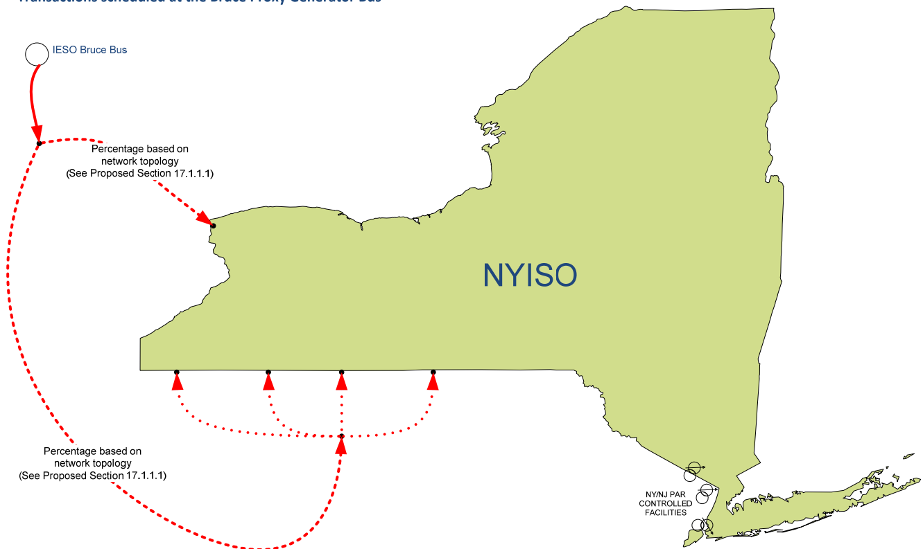
Illustration of Example 1: NYISO's Method of Modeling Power Flows for External Transactions Scheduled at the Bruce Proxy Generator Bus
