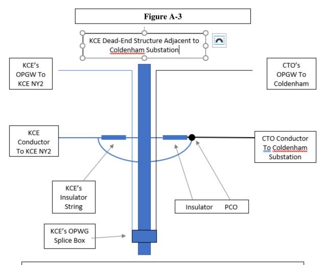
PCO is at the CTO end of jumper loop. OPGW PCO is inside the splice box. Dead-End Tower, Tower Hardware, Insulator Strings, conductor, OPGW and jumper loop between KCE NY2 and the PCO is owned by KCE (shown in blue). Conductor from the PCO and OPGW from the splice box owned by CHG&E (shown in Black)
