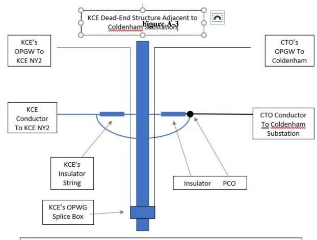
PCO is at the CTO end of jumper loop. OPGW PCO is inside the splice box. Dead-End Tower, Tower Hardware, Insulator Strings, conductor, OPGW and jumper loop between KCE NY2 and the PCO is owned by KCE (shown in blue). Conductor from the PCO and OPGW from the splice box owned by CHG&E (shown in Black)
