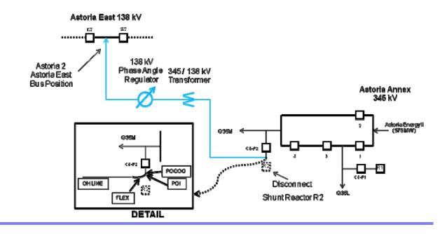
Figure A-1 – Single Line Diagram for Phase 1 System Interconnection
