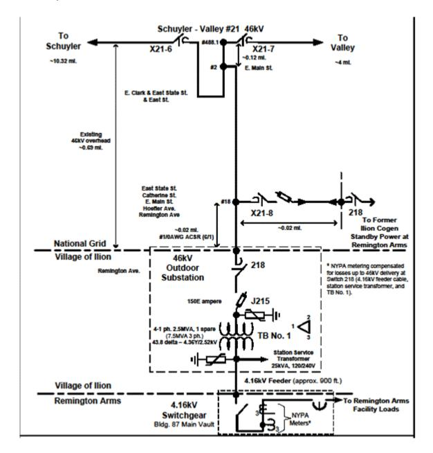
The Transmission Interconnection Point is located at the point where the 46kV tap line serving the Village of Ilion substation interconnects with the Schuyler – Valley #21 line between Switches X21-6 and X21-7 that are integral with National Grid's 46kV EPS.
