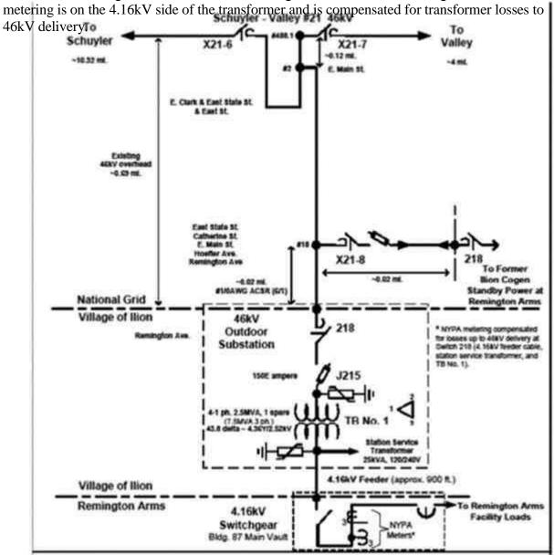
The Transmission Interconnection Point is located at the point where the 46kV tap line serving the Village of Ilion substation interconnects with the Schuyler - Valley #21 line between Switches X21-6 and X21-7 that are integral with National Grid's 46kV EPS.
