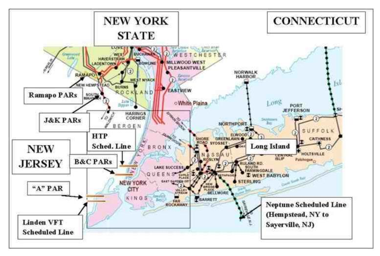
The map above shows that *every* major (230 kV or above) transmission line linking northern New Jersey to New York City or Long Island is managed using a PAR, DC converter, or variable frequency transformer. Neither MISO, nor ITC, has been asked to contribute to the cost of any of the power control devices that are in place at the NYISO/PJM border. Most of the facilities identified on the maps have been in service, reducing loop flows, for years, some for decades.
