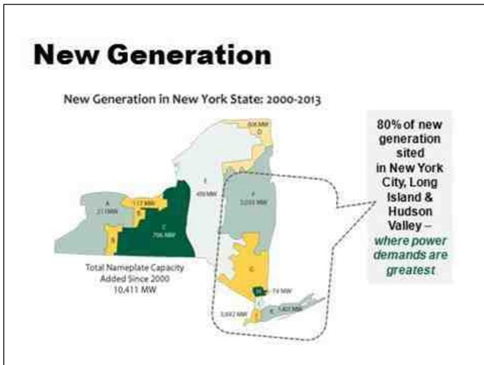
Since the inception of the NYISO, most of the new entrants have been clean, efficient combined cycle units, which has contributed to the New York generation fleet's improved heat rate and reduced harmful emissions. Contributing to this positive environmental trend is the fact that 6,000 MW of older generation has retired or ceased operation since the NYISO's start-up. Old, dirty, and inefficient units will ultimately go away under competition.
