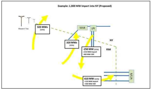
Figure 3: Proposed Protocol - Example of Flows over the ABC Interface, JK Interface, 5018 line and the Western ties
