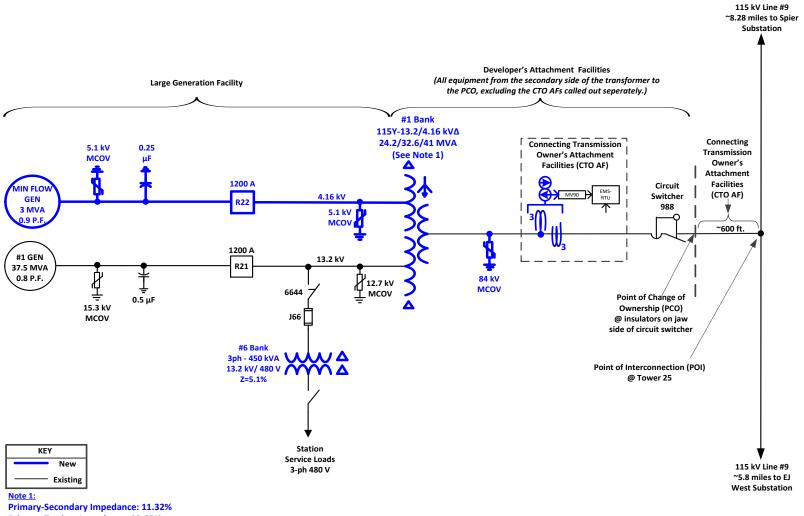
Primary-Secondary Impedance: 11.32% Primary-Tertiary Impedance: 22.65% Secondary-Tertiary Impedance: 10.35%
