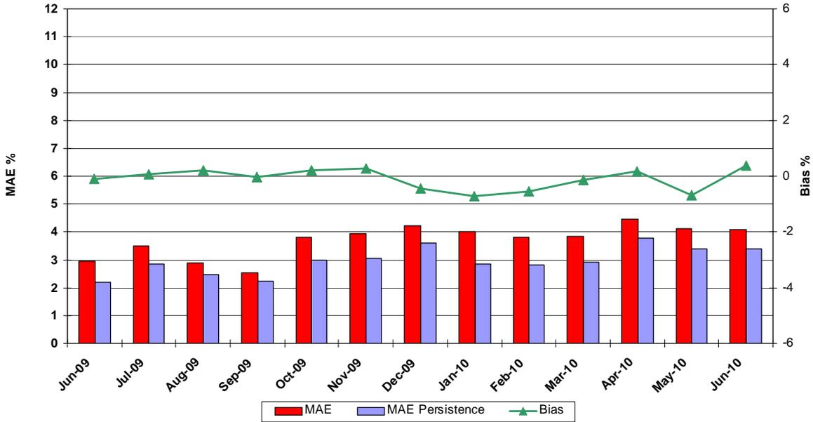
**MAE** - Avg |actual wind generation - hour ahead forecast wind generation| / Wind Capacity
