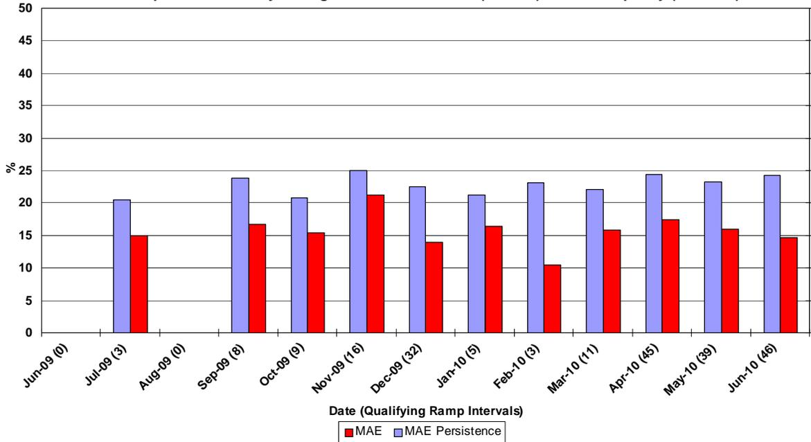
**MAE** - Avg |actual wind generation - hour ahead forecast wind generation| / Wind Capacity
