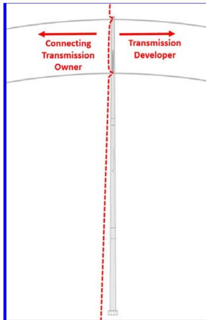
Figure C-3: Representative Substation A-frame Interconnection Drawing
