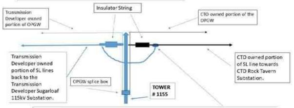
POI at CTO end of jumper loop. OPGW POI is inside splice box. See Detail Box diagram below. Tower, Tower hardware, insulator string on Transmission Developer side of the jumper loops, jumper loops, conductor from the Transmission Developer end of the jumper loops and OPGW splice box and OPGW towards the Sugarloaf 115kV Substation are owned by Transmission Developer.
