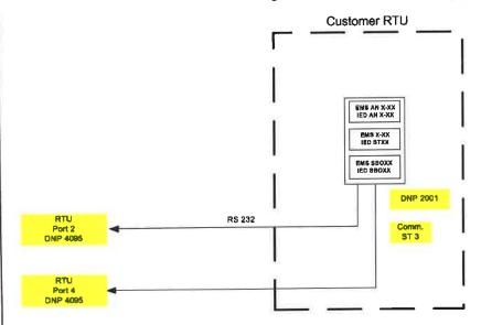
DNP Slave Address: 2001 Baud Rate: 9600 8 bits, 1 Stop, No Parity JMP1-P2=OFF to disable +5V DC RTSCTS=N
